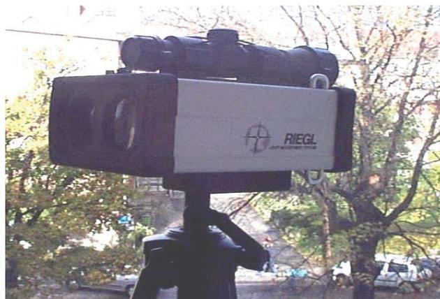
Fig. 9. Laser measurement instrument Riegl LR90-235/P
